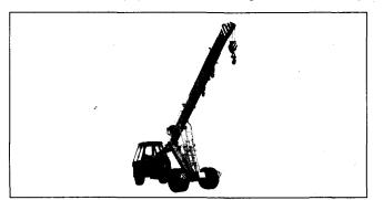
shifting and erecting materials. The Company currently manufactures these cranes of 3 tons to 20 tons capacity. The Company is also in the process of developing 22 ton capacity Crane.
