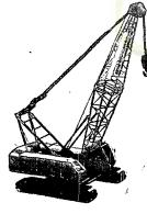
Crawler Cranes are used on soft ground for plant erection and maintenance work or plant renovation. Basically, Crawler Cranes are similar to hydraulic excavators in traction and swing the load at 360 degree. The machine stability is achieved by the tracks themselves.
