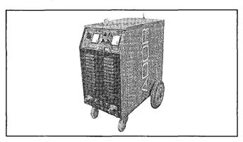
For MMA and TIG process CC mode is selected where, Welding current remains constant in spite of variation in input supply voltage or increase in welding cable length.
