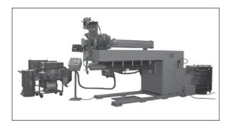
b) Automatic welding of both dished ends using two torches by the press of single button. Can also do 2 runs of welding Non-stop, with manual removal of the slag.
