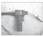
It has swan neck which can be rotated in 360 degree for ease of welder to weld the job in any position.
