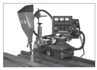
It is the unique Mechanization attachment mounted on travel carriage for GMAW / FCAW / SAW welding using standard CO2 Welding machine, which is very useful and handy to complete GMAW / FCAW / SAW jobs without really purchasing the complete SAW welding outfit consisting of power source and welding head.
