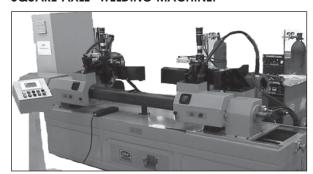
This is a 5 servo controller mechanism suitable for square & round axle of following specifications:
