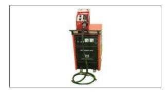
RANGER-403 is a thyristor based MIG / MAG outfit suitable for heavy fabrications like ship building industry. Power source of this outfit is a light weight and compact design in thyristorised models. It has wirespeed and voltage adjustment on the wire feeders which gives easy access to welders for parameter adjustment during welding.
