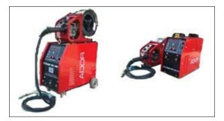
These are new high efficient and high power factor IGBT based GMAW welding outfits, suitable for continuous wire welding application with various types of material and active and inert gases. The complete system consists of power source, wire feeder, MIG torch and interconnecting cables.
