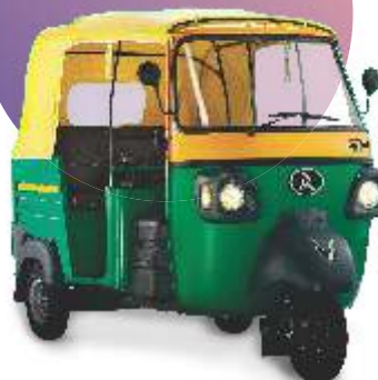
REAR ENGINE PASSENGER 3+1 CNG
