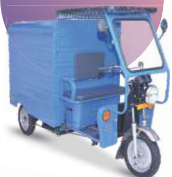
ATUL ELITE DELIVERY VAN MOTOR POWER 850/1000 W 350 KG PAYLOAD CAPACITY
