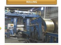
Both HOT rolling and COLD rolling facilities. Mesta Hot Rolling mill to produce Hot roll billets with thickness ranging 170mm to 16mm. High speed reversible 4 Hi Mills and Modern 20 Hi Cluster Mills with automatic gauge control.
