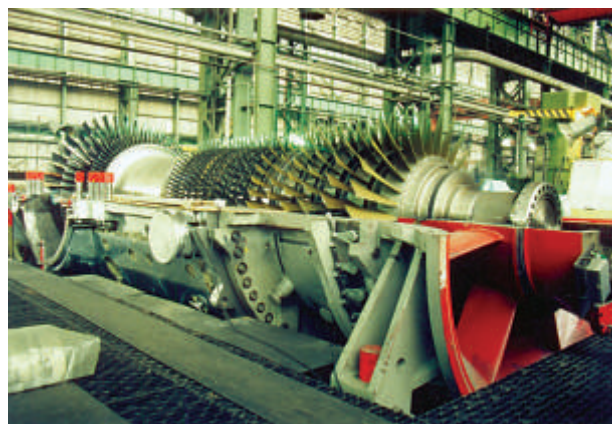
159 MW Gas Turbine on assembly bed
