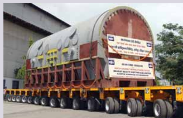
600 MW Turbo-Generator being dispatched for North Chennai TPS
