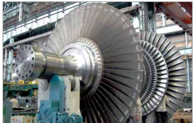
660 MW Turbine LP Rotor for Bara Project, under assembly at HEPP, Haridwar
