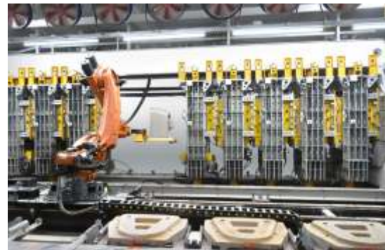
Sanitaryware Robotic Pressure Casting For producing clone type product every time
