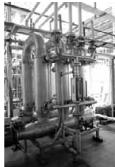
The ceramic based ultra filtration unit, at the Ankleshwar API plant, is the first of its kind in India for effluent treatment
