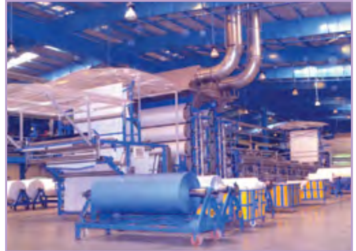
Pad steam dyeing range-versatile fabric processing machine with advance dyeing features
