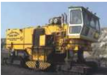
India's 1st indigenous Surface Miner powered by Cummins KTA-38-C
