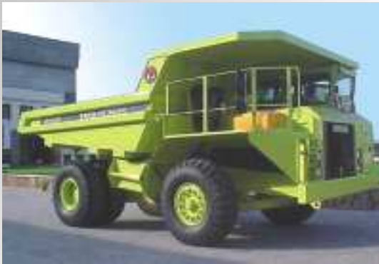
35T Dump Truck powered by Cummins N-14-C
