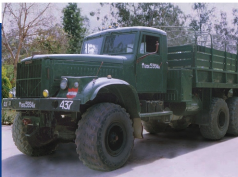
Kraz 255 Defence Truck repowered by Cummins NT-743-C
