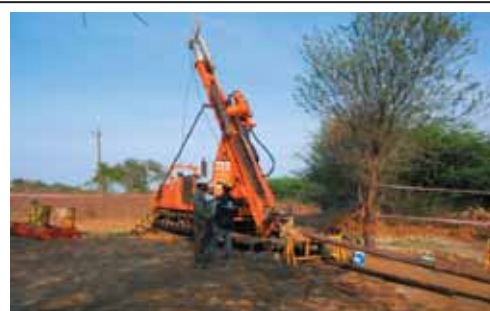
Fig-8 : Diamond Core Drilling operation at Ganajur Main Prospect, Ganajur-Karaji PL.
