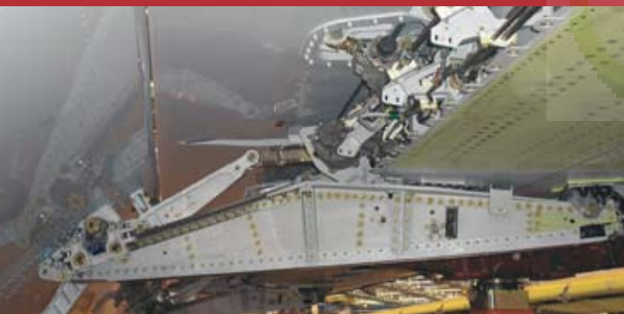
The Airbus 320 Flap-Track Beam that will be assembled by Dynamatic Aerospace®, Bangalore
