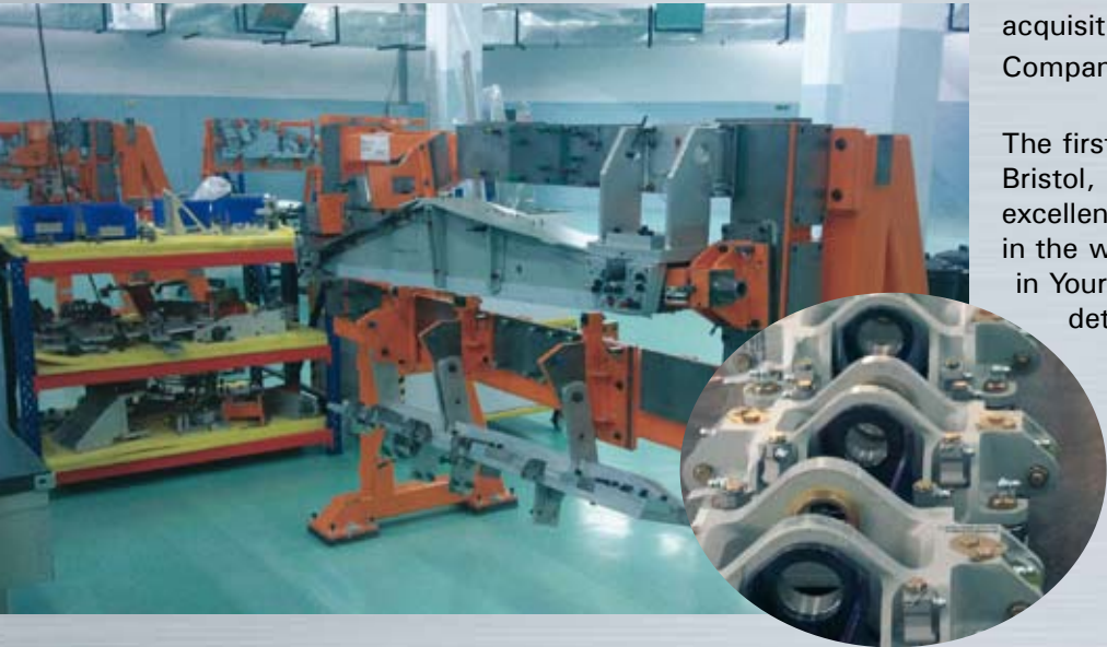
The Airbus A320 Flap-Track Beam under production at 'Prana', Dynamatic®'s new Aerospace facility
