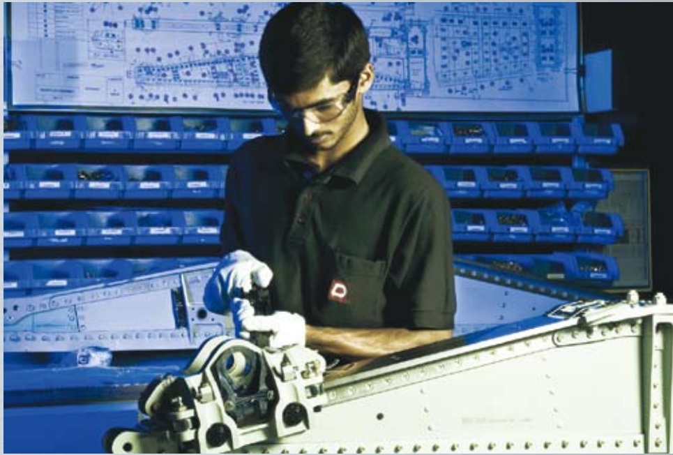
Carriage Assembly on a Flap Track Beam for the Airbus A320 Single Aisle Aircraft at Prana, Dynamic Aerospace®
