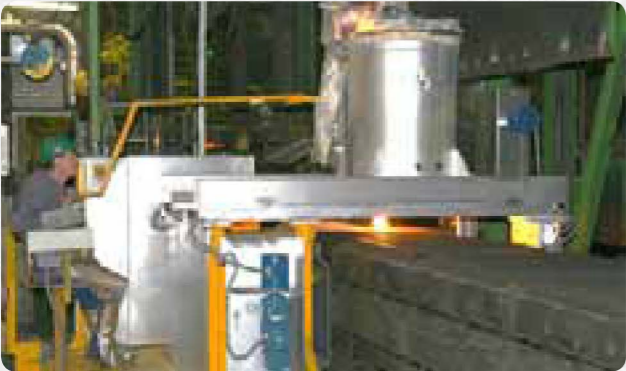
A new pouring machine for steel castings was installed into series process of the GFD moulding line at Eisenwerk Erla GmbH
