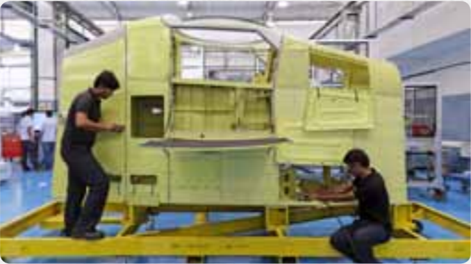
Aft Pylon Assembly and Cargo Ramp Assembly for the Boeing Chinook CH-47F Helicopter at Dynamatic Park, Bangalore
