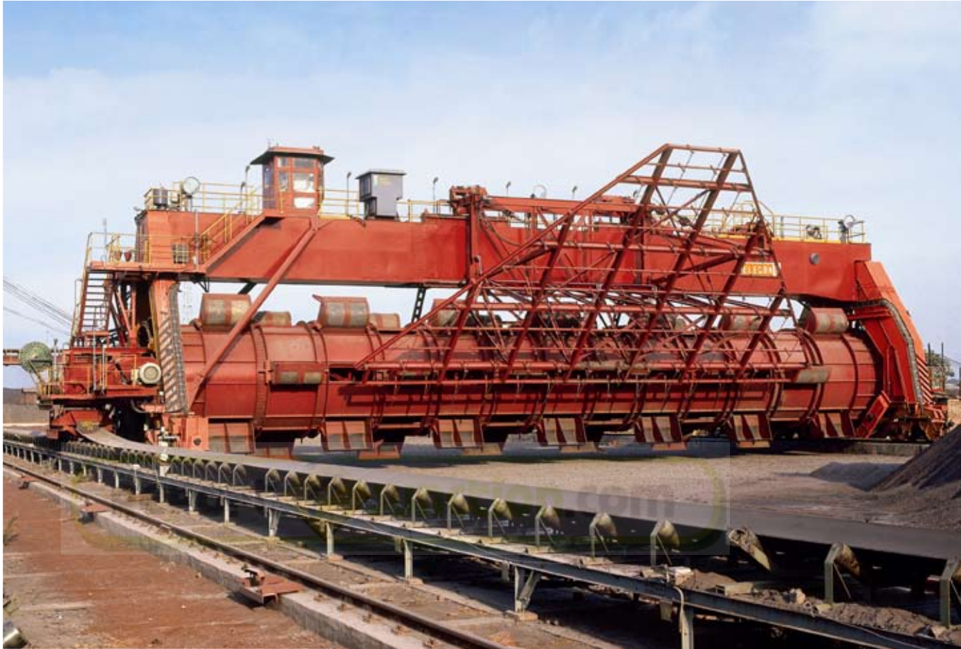
Barrel-type blender reclaimer
