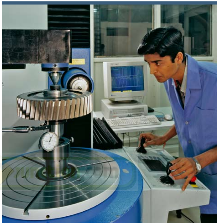
Gear tooth profile tester
