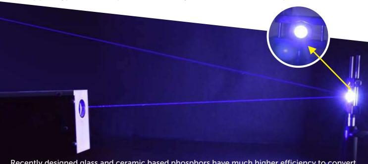
Recently designed glass and ceramic based phosphors have much higher efficiency to convert blue laser light to white light.
