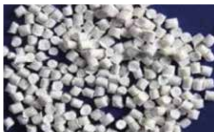
Polyester Chips: Industrial intermediate product used to manufacture Polyester Yarn.
