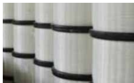
Monofilament Yarns: Superior technology from Reifenhäuser GmbH, Germany. Used in zippers, fishing nets, sports strings, magic fasteners etc.
