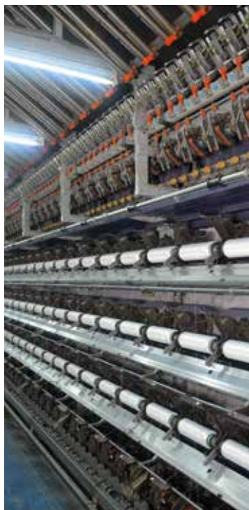
Polyester Partially Oriented Yarns (POY): Intermediate product, post Texturizing used for producing all kinds of Fabrics.
