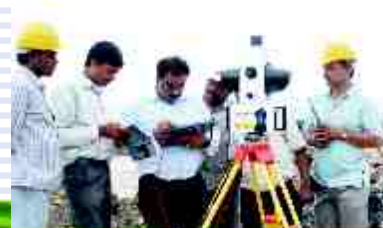
State-of-the-Art Laser 3D Scanner being used for Mine Planning, Monitoring, Design and Volume of Rock / Ore estimation
