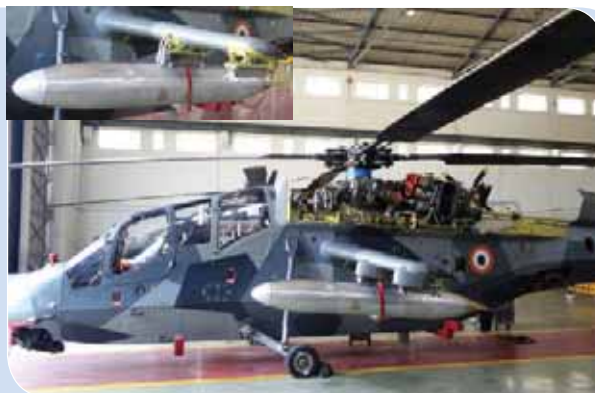
Auxiliary Fuel Tank Integrated on Light Combat Helicopter.
