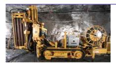
**V30 Slot Machine** Enables long slot raising.
