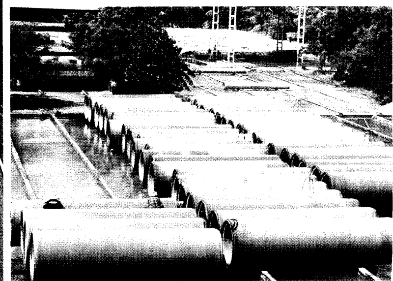
Prestressed Concrete Cylinder pipes in yard at Thanjavur factory
