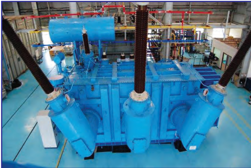
55MVA, 400/11.5 KV, Start up Transformers
