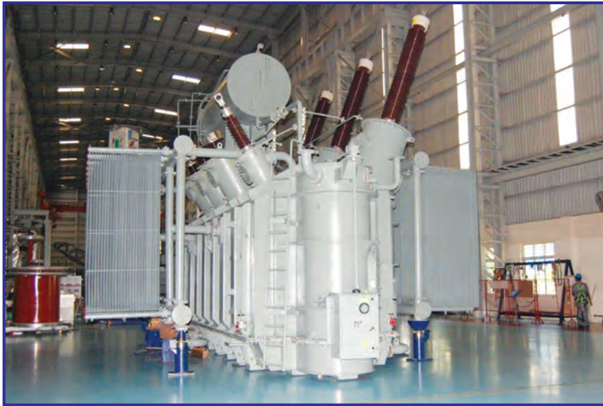
180MVA, 235/13.8 KV, Generator Transformers
