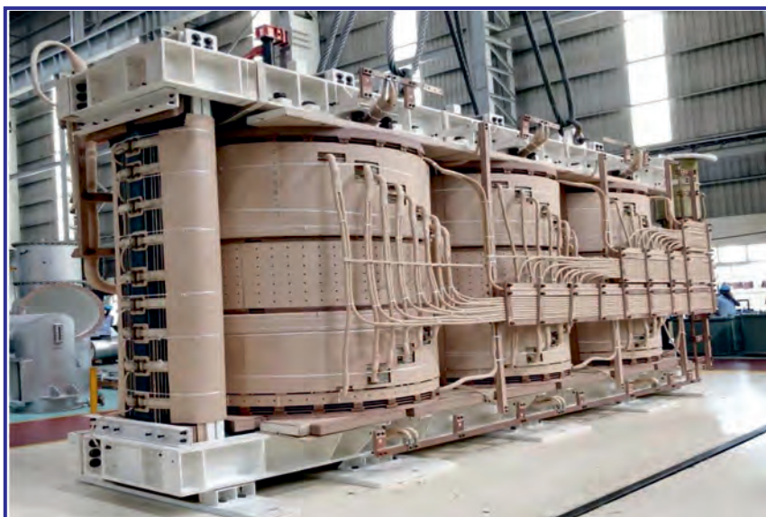
Internal assembly of 150 MVA, 220 kV Transformer: Performance coupled with aesthetics
