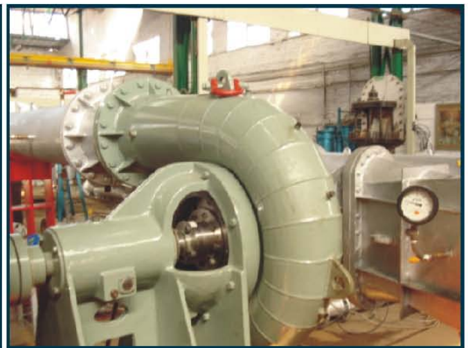
Actual Model Test of Metallic Volute Pumps at Jyoti Test Laboratory.
