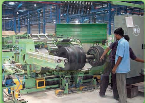
Green Tyre Assembly in Progress
