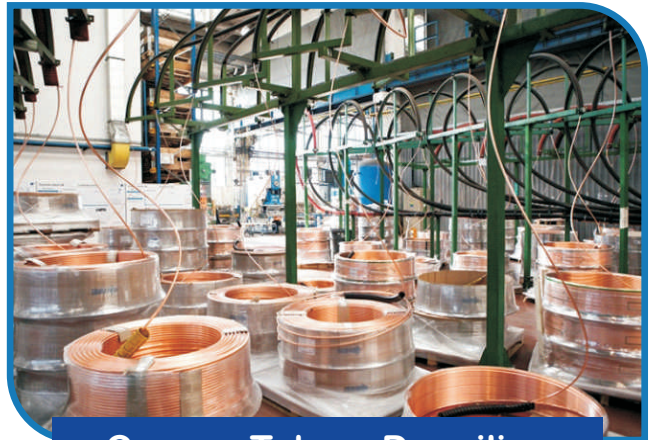
Copper Tubes- Decoiling of raw material
