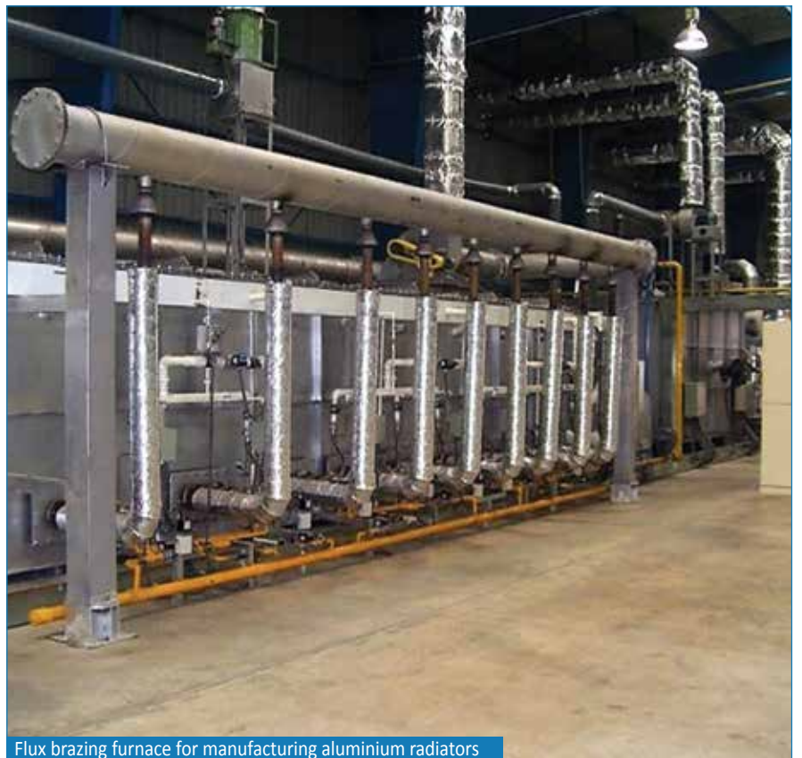
Flux brazing furnace for manufacturing aluminium radiators
