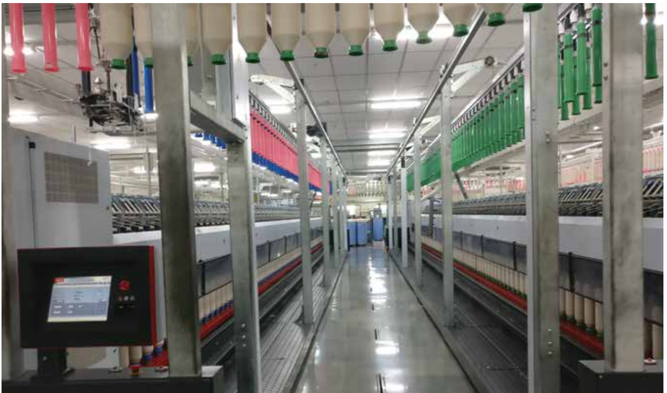
Zinser - 5 A Speed Frames with Auto doffing
