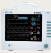
These are used in operation theatres & intensive care units. These systems are used for monitoring the patient's vital signs such as ECG, blood pressure, temperature & oxygen level saturations.
