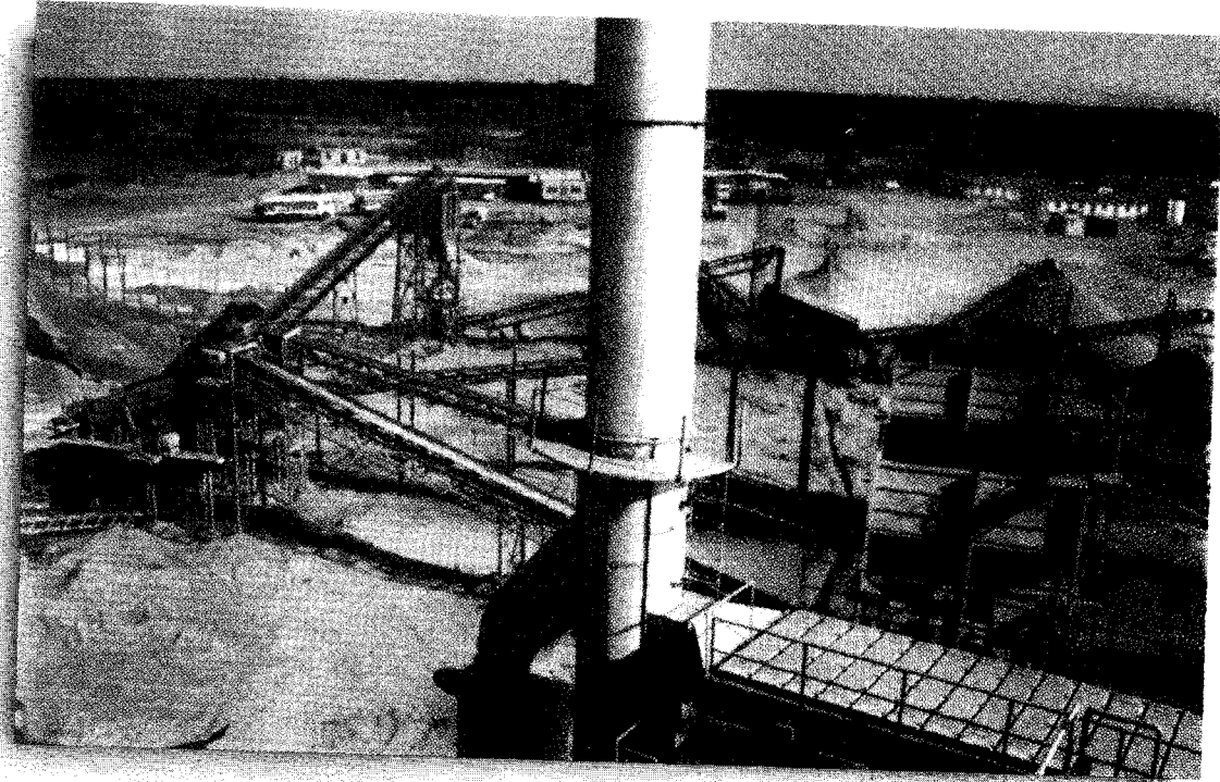
▲ 200 M/T Stone crushing unit per hour at Udaipur Project
