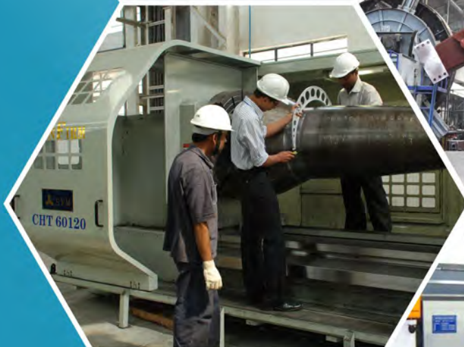
Axle pin part (SG Iron Casting) for wind turbine
