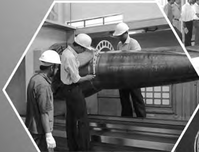
Axle pin part (SG Iron Casting) for wind turbine
