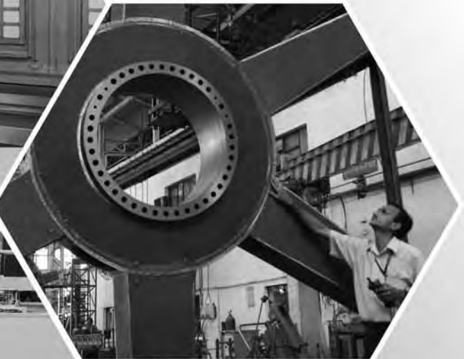
Manufacturing of Stator Carrier of Wind Turbine parts
