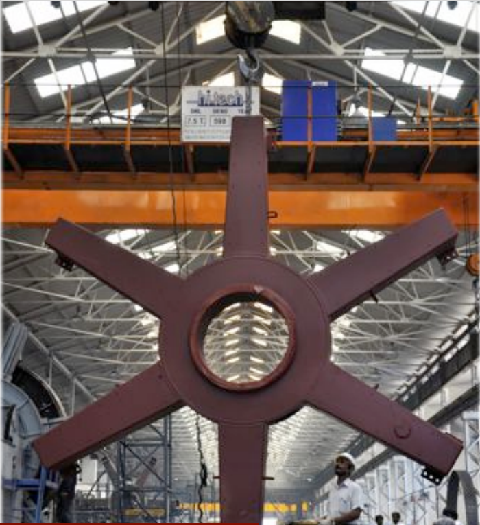
▼ Wind turbine stator carrier : Finished Weight 2177 kgs
