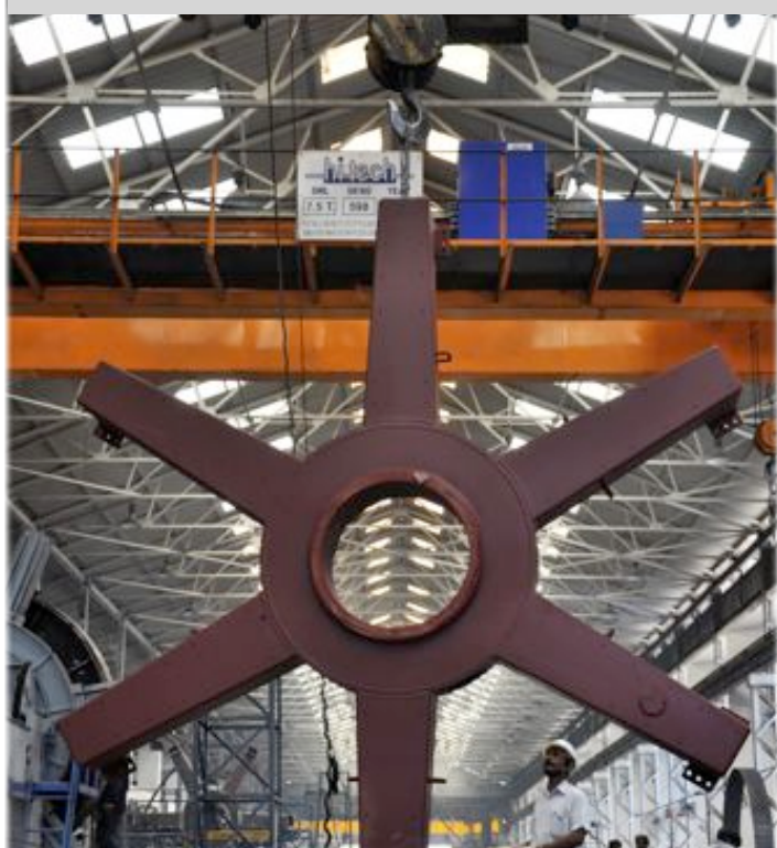
▼ Wind turbine stator carrier : Finished Weight 2177 kgs
