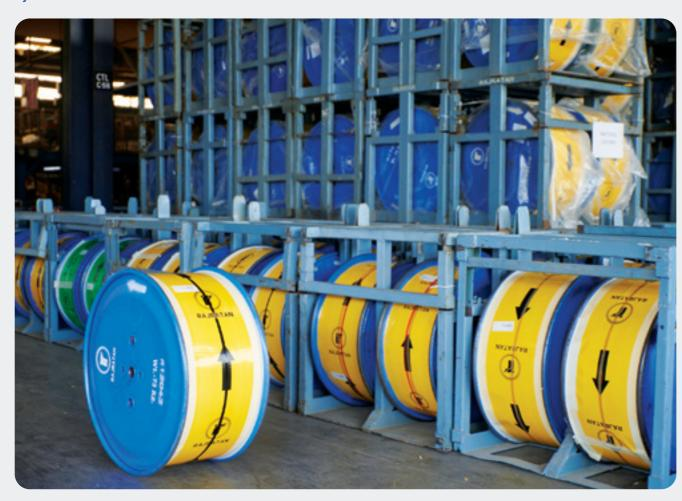
It is also known as re-enforcement wire, and its purpose is to hold the tyre to the rim of the wheel while resisting the constant push of inflated pressure. Bead wire is the critical link that transfers the vehicle load from the rim to the tyre, preventing vibration while driving.
