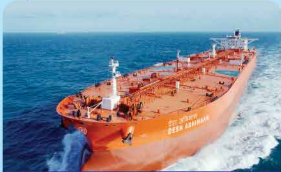
The Shipping Corporation of India Ltd. acquired secondhand Suezmax Tanker M.T. Desh Abhimaan to its fleet on 26th April, 2017. The vessel has a gross tonnage of 81084 and deadweight of 158710 tonnes.
