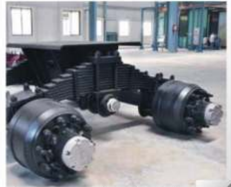
Bogie suspension for heavy duty Trailers
