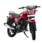
The Company introduced TVS JIVE 110 cc with innovative T-Matic technology in the executive segment which accounts for 60% of the total motorcycle market. This motorcycle allows hands-free gear shift because of absence of the clutch lever. Coupled with this an anti-stall mechanism makes smooth riding possible at low
