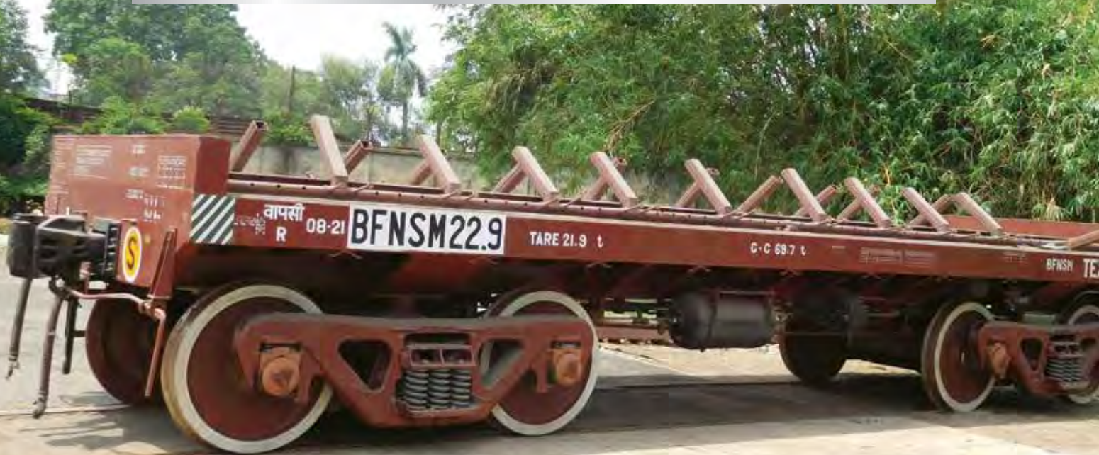
New Design Flat Steel Wagon 'BFNSM' for transportation of Steel Coils
