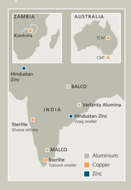
Sterlite is principally a copper smelting and refining business in India with two small copper mines in Australia. The capacity at Tuticorin smelter was increased in April 2005 from 180,000 tpa to 300,000 tpa. The output is refined into copper cathode and rod at Tuticorin and Silvassa.
