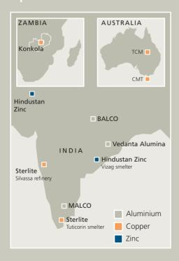
Sterlite is principally a copper smelting and refining business in India with two small copper mines in Australia. The capacity at Tuticorin smelter was increased in April 2005 from 180,000 tpa to 300,000 tpa. The output is refined into copper cathode and rod at Tuticorin and Silvassa.
