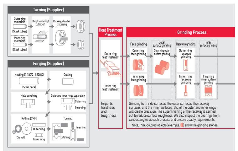
Process into a ring shape by turning or forging the steel tubes, and turn the raceway and the inner surface of the rings [both outer and inner rings].
